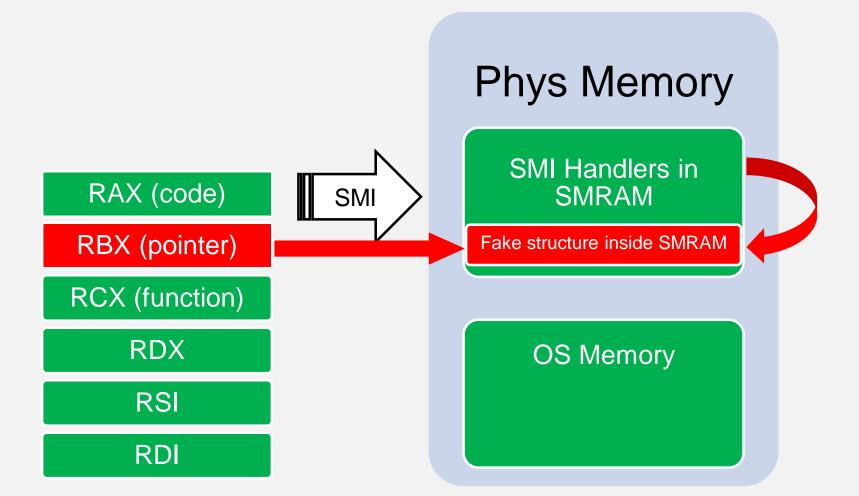
Exploit tricks SMI handler to write to an address inside SMRAM Attacking and Defending BIOS in 2015
