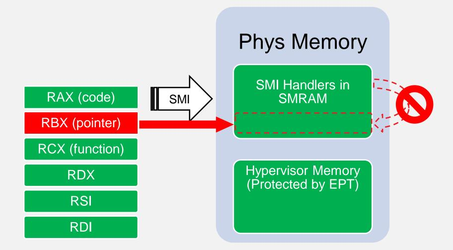
Firmware SMI handler validates input pointers to ensure they are outside of SMRAM preventing overwrite of SMI code/data
