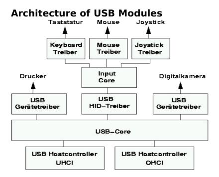
hid.o (HID = Human Interface Device) and input.o (Input Core) are only for a USB keyboard (usbkbd.o), Mouse (usbmouse.o) or Joystick otherwise they are not needed.
