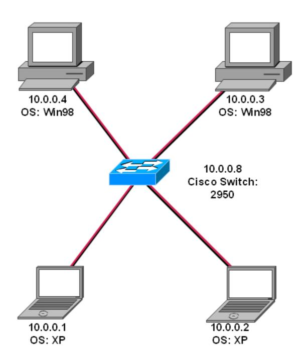
Well this was our test setup as you can see we used a cisco switch to do the packet switching and 2 lab comp together with our notebooks.
