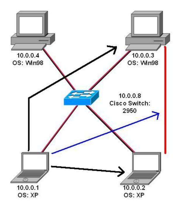
The blue arrow indicates what we want to sniff. The black arrows indicate what we are going to poison. So we fired C&A\* up and started to scan for the MAC addresses.
