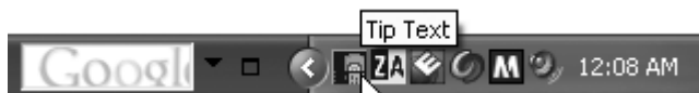
Figure 4-5. Showing the icon and tool tip for a new system tray application
