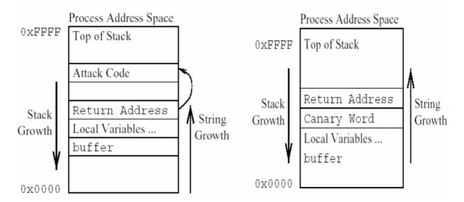
Fig 2.3 : Stack Smashing Buffer Overflow Attack
