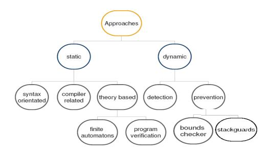
Fig 2.1 : Classification of approaches undertaken against buffer overflow
