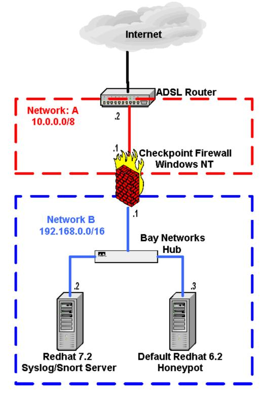
The firewall is a Windows NT machine running Checkpoint FW-1, this machine controlled who had access to which parts of the network. The set-up is very simple:-
