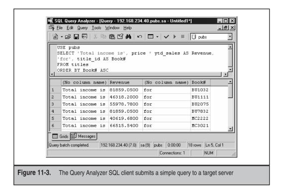
Query Analyzer can be used to connect to SQL Server, guess passwords, and perform simple manipulations of server data and configuration parameters, all from an easy-to-use graphical interface.
