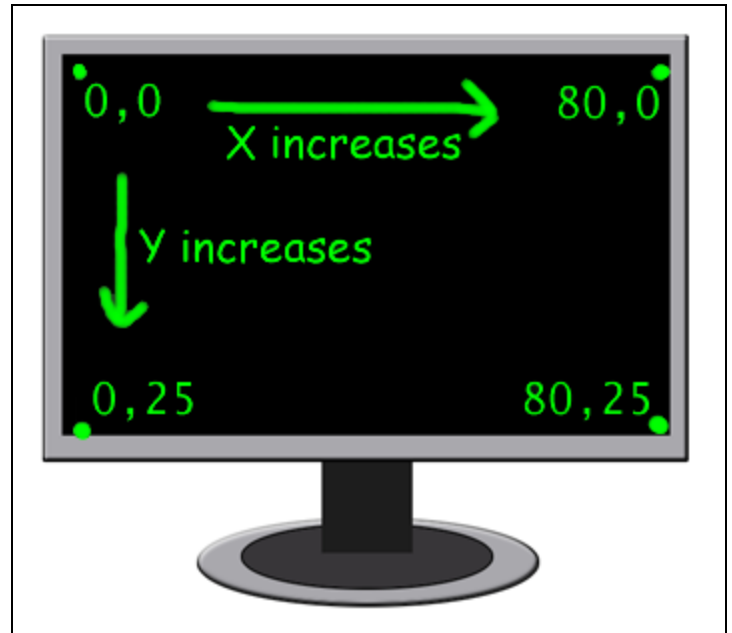
Figure 11-12: The Cartesian coordinate system on a computer monitor.
