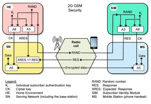
Figure 1. Security architecture in 2G GSM
