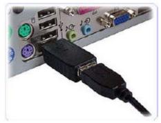
Figure 5: USB Keylogger (Keelogger)
