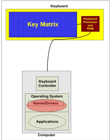
Figure 3: Kernel-based Keylogger
