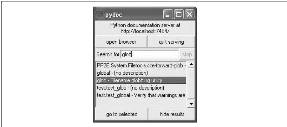
Figure 14-1. The Pydoc top-level search engine GUI: type a name of a module you want documentation for, press Enter, select the module, and then press “go to selected” (or use no module name, and press “open browser” to see all available modules).
