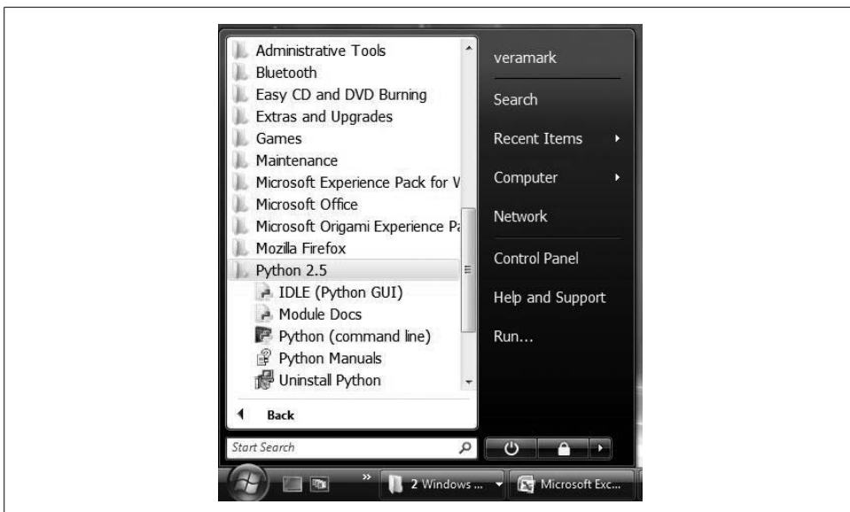
Figure 2-1. When installed on Windows, this is how Python shows up in your Start button menu. This can vary a bit from release to release, but IDLE starts a development GUI, and Python starts a simple interactive session. Also, here are the standard manuals, and the Pydoc documentation engine (Module Docs).
