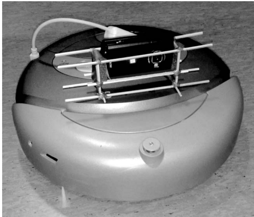
Figure 11.12 Nokia N80 mounted on a Roomba robotic vacuum cleaner
