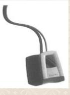
Figure 3.9: Compaq Fingerprint Identification Technology Source: Compaq Computer Corporation
