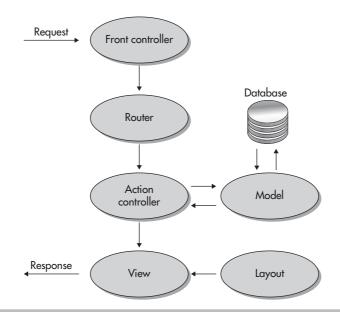
Figure 2-1 Interaction between models, views, and controllers
