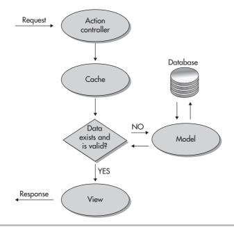
Figure 12-8 Flow chart of cache operation
