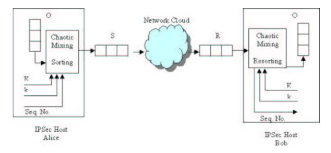
Figure 4.7: Block diagram of sorting and resorting process
