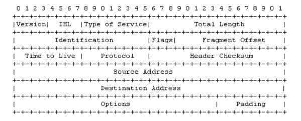
Figure 3.2: The IP header
