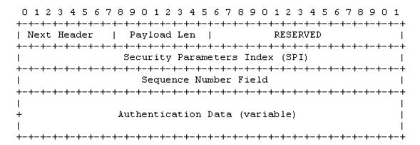
Figure 4.1: The AH header
