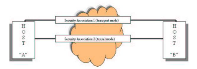
Figure 4.3: End-to-end security between two hosts.
