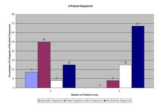
Figure 4.13: 4-packet sequence against different position errors
