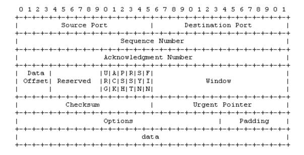
Figure 3.1: The TCP header
