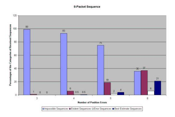
Figure 4.18: 8-Packet Sequence against different position errors
