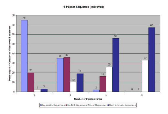
Figure 4.16: 6-Packet (improved) sequence against different position errors
