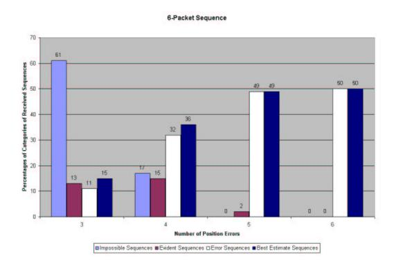
Figure 4.15: 6-packet sequence against different position errors
