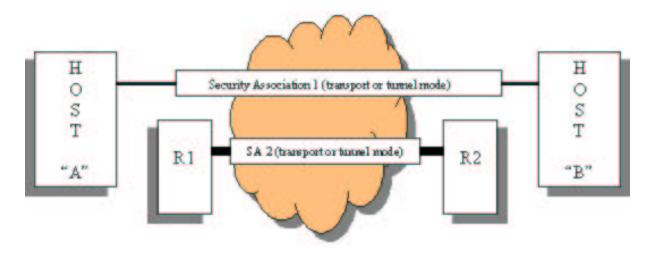
Figure 4.5: The complete end-to-end scenario involving IPSec implemented intermediate nodes
