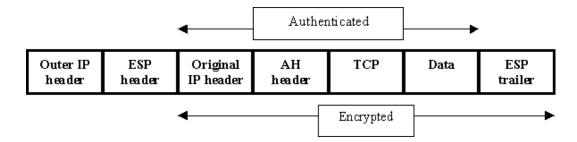
Figure 6.1: AH in transport mode and ESP in tunnel mode
