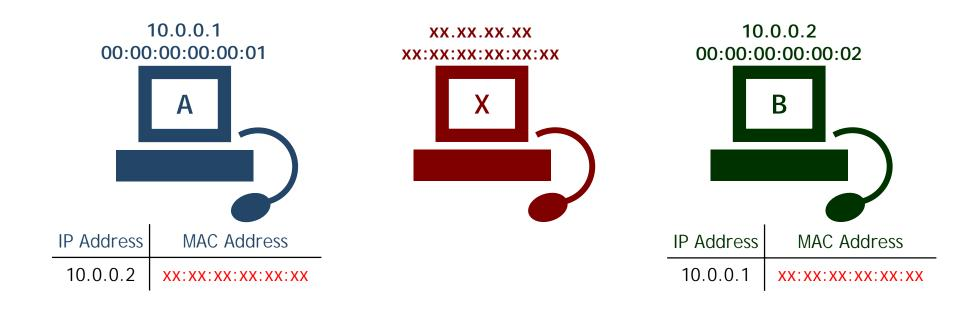
Computer X needs to do one more thing to prevent disrupting the communication Between A and B. It must forward the packets A sends to B on, and visa versa.
