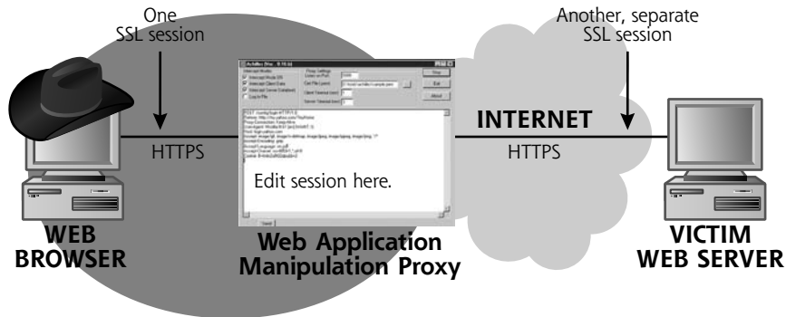
Figure 7.33 Handling HTTPS (that is, HTTP over SSL) with a Web application manipulation proxy.
