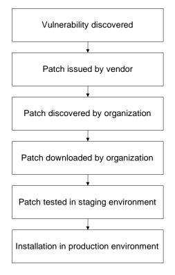
Figure 2: The patch latency stages
