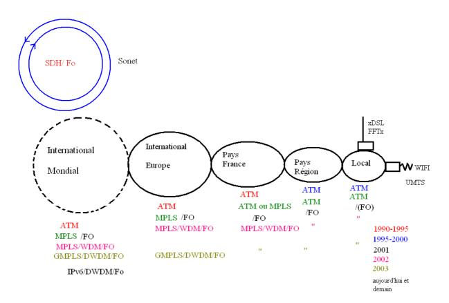
**ATM**: Asynchronous Transfert Mode **MPLS**: Multi Protocol Label Switching
