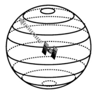
Figure 1.4: Surfaces of Position for Range Measurements.
