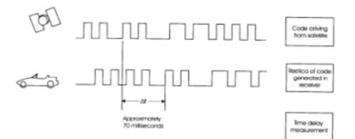
Figure 1.8: One-Way Ranging Using PRN Codes.
