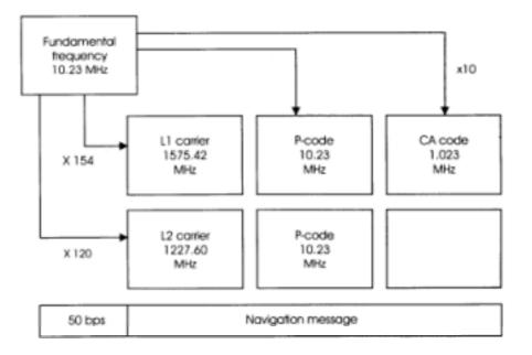
Figure 1.2: GPS Satellite Signal Components.
