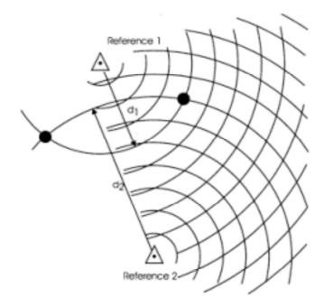
Figure 1.5: The Intersection of Circular Lines of Position for 2-D Positioning.
