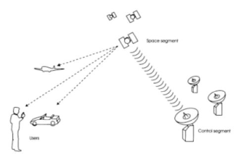
Figure 1.1: GPS System Elements.
