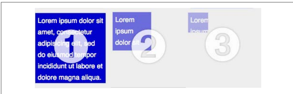
Figure 7-1. Passing a speed in to the show method animates height, width, padding, margin, and opacity
