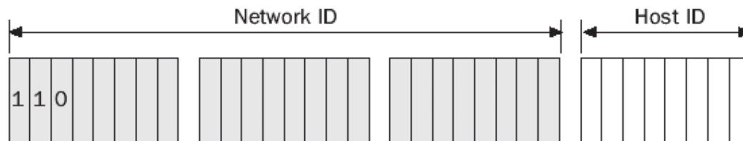
Figure 6-6. The class C address showing the network ID and the host ID.
