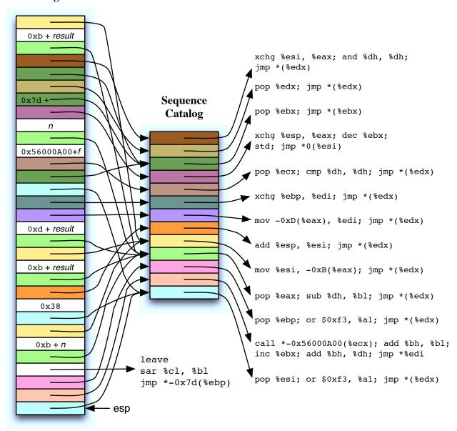
**Figure 4:** Function call gadget. This convoluted gadget makes the function call  $result \leftarrow f(arg_1, arg_2, \dots, arg_k)$  where the arguments have already been placed at  $n+4, n+8, \dots, n+4k$ . The return value is stored into memory at address result.
