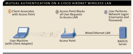
**MUTUALLY SECURE:** The client authenticates the network via a RADIUS server; likewise, the RADIUS server authenticates the client. The two sides of the authentication scheme are decoupled on separate secure channels, with the access point in the middle.
