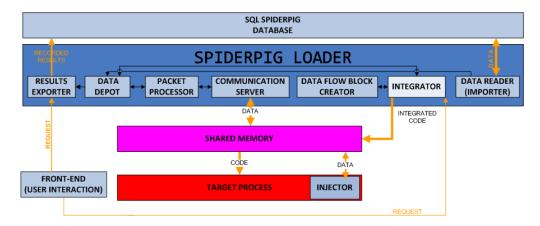
Figure 3: Internal structure of *SpiderPig Loader Module* with marked directions of the data flow.
