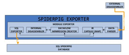
Figure 2: Internal structure of *SpiderPig Exporter Module* with marked directions of the data flow.
