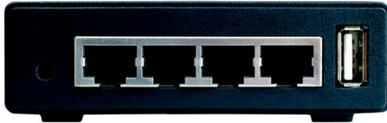
Figure 2-1: USB PrintServer's Back Panel
