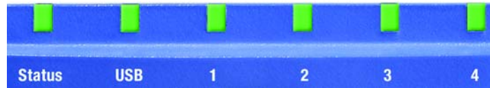
Figure 2-2: The USB PrintServer's Front Panel
