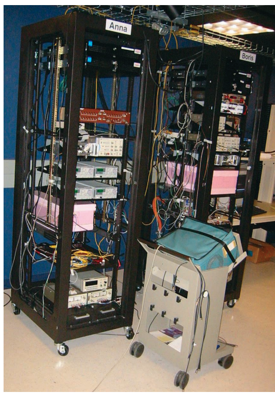
Figure 2. BBN quantum cryptography system (Anna and Boris). A full-featured quantum cryptography system now operating in the world's first quantum cryptographic network, under the streets of Cambridge, Massachusetts.
