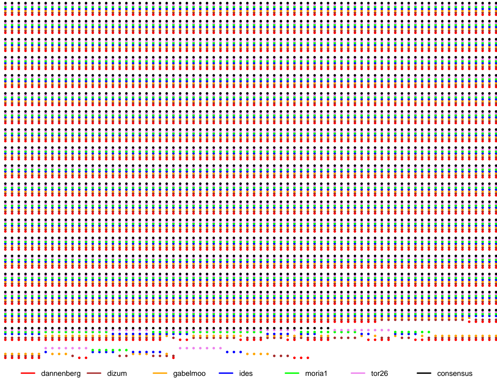
Figure 1: The Running flag shows how the voting process should work. Most relays are included in all six votes (colored dots) and therefore in the consensus, too (black dots). In the third from last row, relays are missing in single votes which does not affect the consensus. In the last but one row, relays are missing in three or more votes and are therefore not included in the consensus.
