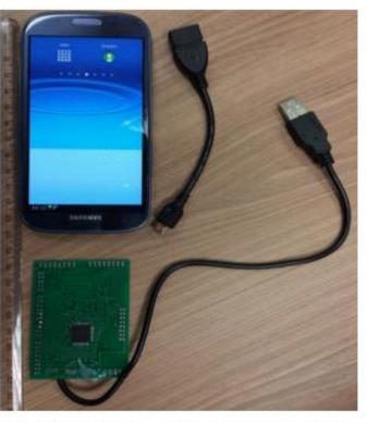
The attackers responsible for this "black box" ATM hack relied on a mobile device and a USB-based circuit board.
