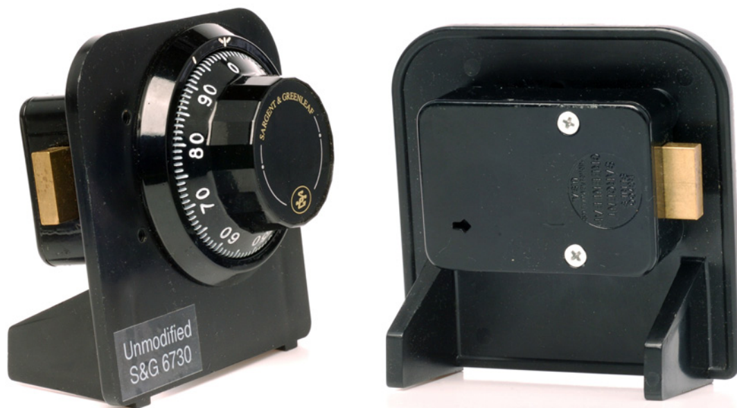
Figure 1: Standard lock package (in this case, a Sargent & Greenleaf model R6730), shown mounted on a display stand. The dial (left image) is accessible on the outside of the container. The internal lock module (right image), in a standard form factor, contains the lock mechanism and retractable lock bolt (the brass tab at the far right). Note the change key hole on the back of the lock case, into which the user can insert a tool to change the combination when the container is open. The dial is connected to the lock module via a spindle running through a small hole in the container wall.
