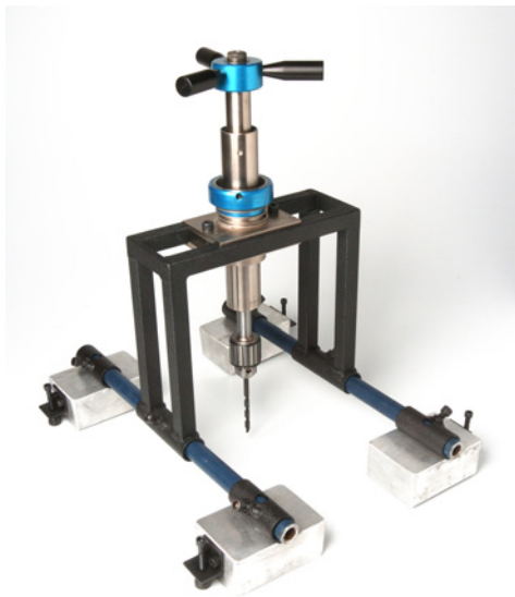
Figure 12: A portable drill rig designed for safes and vaults. As shown, the base is attached to the side of the container by powerful permanent magnets; it can also be attached with machine screws or nylon straps. An ordinary low- or medium- speed handheld electric drill (not shown) supplies power.
