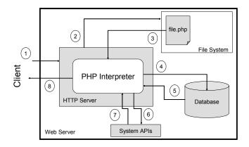
Figure 1. Typical web application architecture
