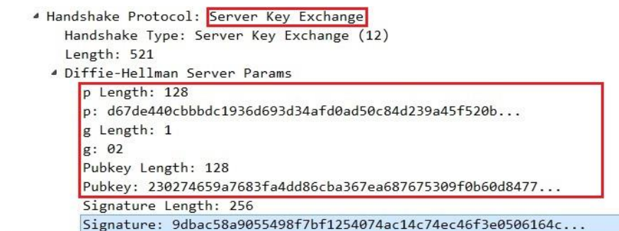
Figure 5 – Server Params Structure from TLS Server Key Exchange Message
