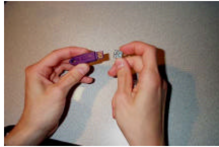
Figure 4b: Removal of the metal USB housing.
