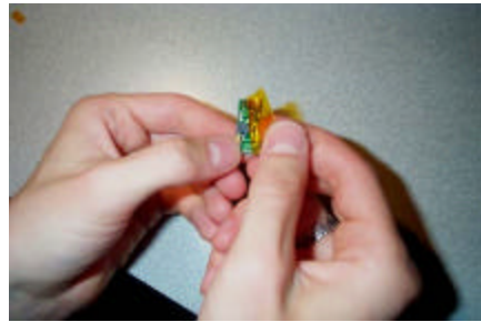
Figure 4f: Removal of tape wrapped around the circuit board. This may be a tamper-detection attempt, but the lack of tape is not visible when the device is properly closed.
