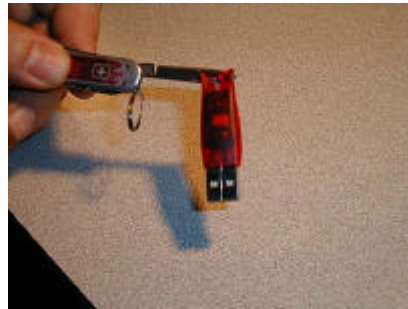
Figure 2b: Using a knife to pry open the tail of the housing. This gives an entry point to pry open the side of the housing.
