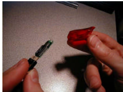
Figure 2d: Successful penetration of the housing and easy removal of the key's circuit board.
