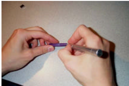
Figure 4c: Prying of the plastic housing.
