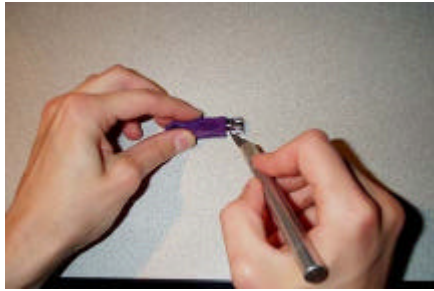
Figure 4a: Lifting the four tabs of the metal USB housing.
