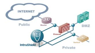
The IntruShield architecture also enables IDS systems to become integral to High Availability topologies (active-active or active-passive) and asymmetrically routed deployments. Here IntruShield systems can fail over to a hot standby.
