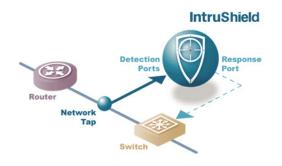
*In-Line Mode:* IntruShield systems sit in the data path, with active traffic passing through them. The IntruShield system prevents network attacks by dropping malicious traffic in real time. Preventative action can be custom-defined at a highly granular level, including automated dropping of DoS traffic intended for a specific Web server. Wire speed prevention and highly available operation enable IntruShield system deployment in mission-critical environments.
