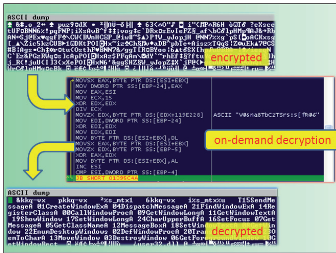
Figure 2: Part of the on-demand decryption algorithm with sample encrypted and decrypted strings.
